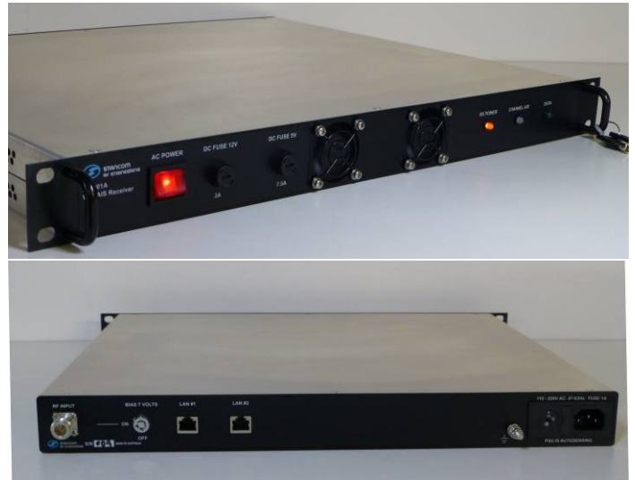
Figure 1- AIS001 Under operation
