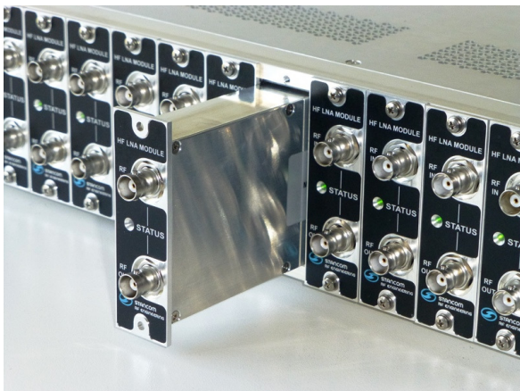
Figure 2 – Easy module removal
